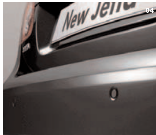
04-06 The Sensor pack includes ultrasonic front and rear parking sensors which omit an audible warning as objects become closer, cruise control (standard on the Comfortline) which can maintain a constant speed from 20 mph upwards and automatically switches off when the brake or clutch is engaged and an electronic tyre pressure monitoring system which alerts you should a tyre lose pressure. Optional on all models.
