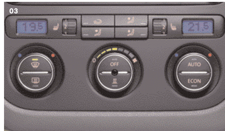
03 The 2Zone electronic climate control is fully automatic to retain a precise internal temperature. It also benefits from a twin zone setting that allows the driver and front passenger up to 4°C difference in their chosen temperature settings. Optional on all models.
