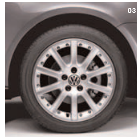
03 'Grand Prix' design 7J x 17 alloy wheels with 225/45 R17 tyres, anti-theft wheel bolts and a steel space saver spare wheel. Optional on all models.
